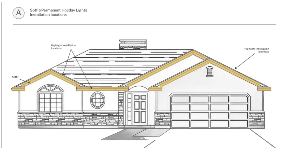
Figure 4 | Permanent holiday lighting must be installed along the soffit line and visually integrated with the residence.
